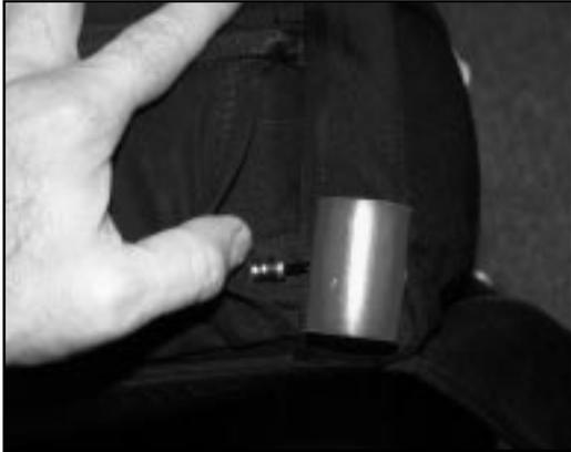
Feed ripcord into housing inside BOC pouch opening. [Fig.1]
