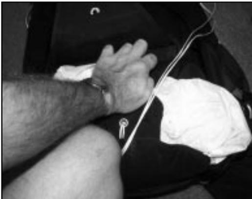
Thread pull-up cord up through center of main spring and through grommet in the top of main PC. Depress spring and pull fabric from coils. [Fig. 3]
